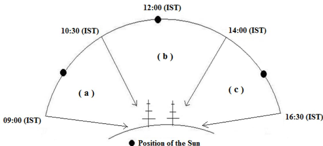
Figure 2. Reveals how the two LPDAs are used as anti-sunward detector during (a) 09:00 hrs to 10:30 hrs of IST and (c) 14:00 hrs to 16:30 hrs of IST whereas sun-ward detector during (b) 10:30 hrs to 14:00 hrs of IST.
