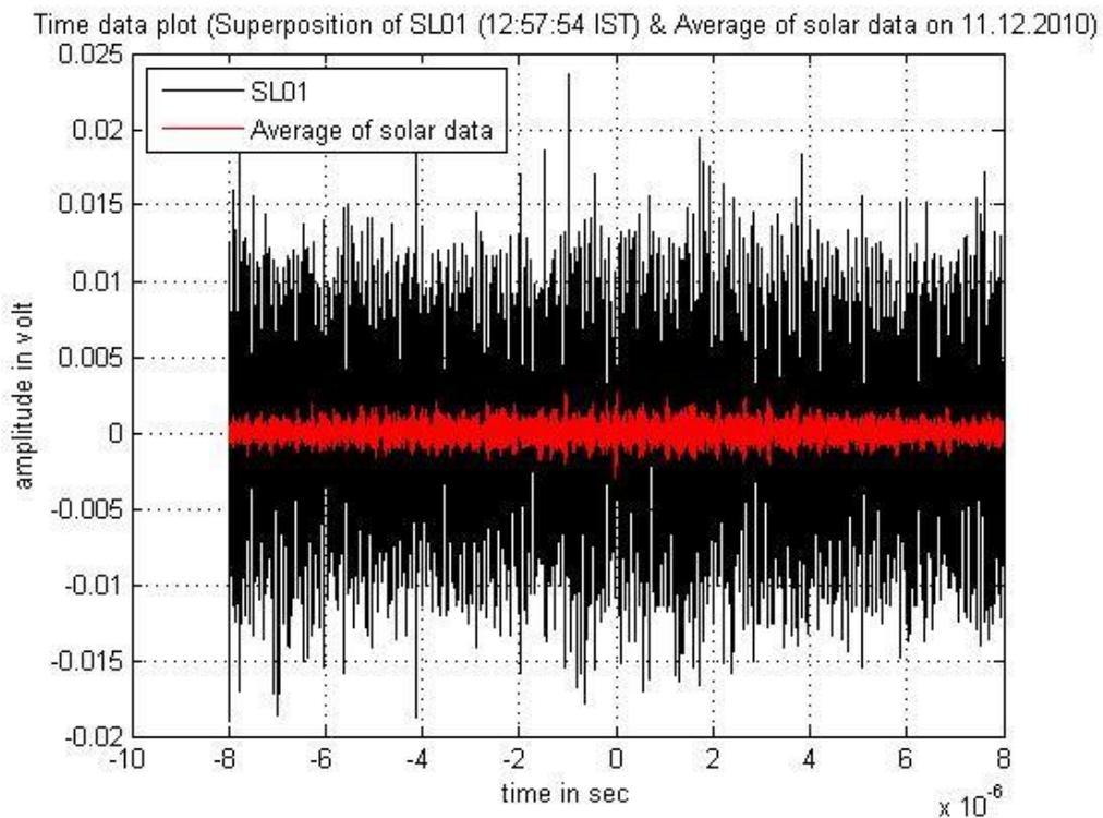
Figure 7. Superposition of time-voltage plot of average solar data and solar data which contain expected solar bursts.
